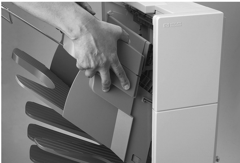
Figure 6-180 Mailbox with Stapler, Stapler Removal or Installation
